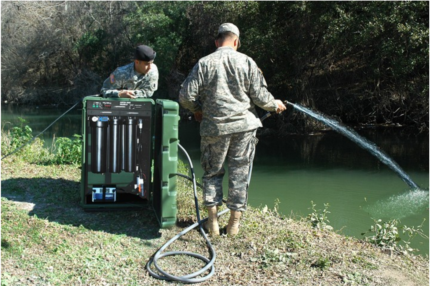
Aspen 5500M Water Purification System on Natural Stream
