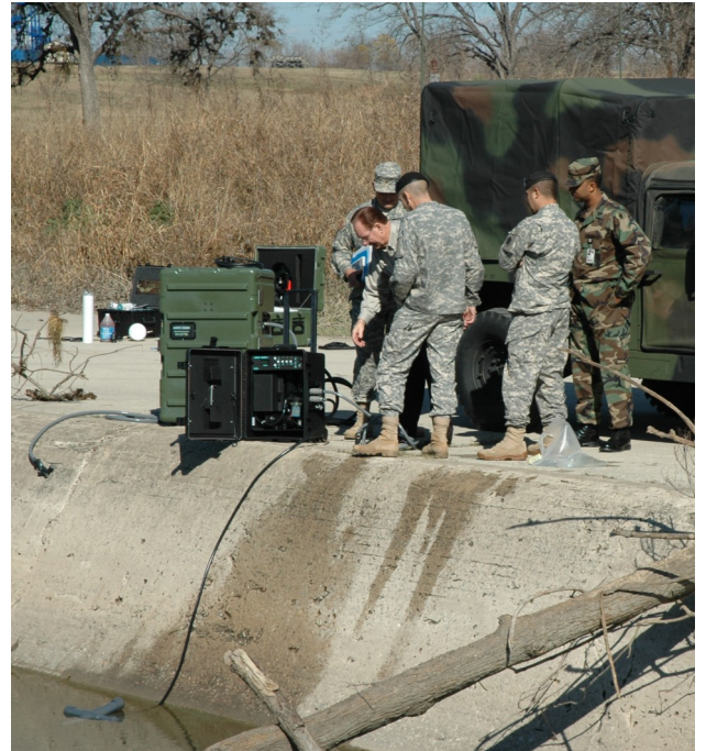
Aspen 1800BC Water Purification System on Drainage Ditch
