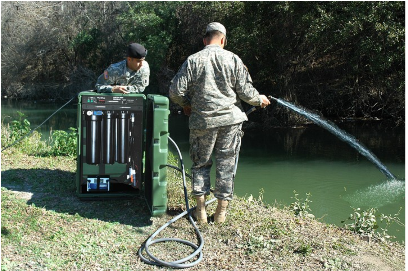
Aspen Water Purification System on Natural Stream
