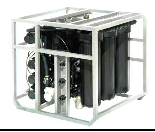
The ASPEN 1500RO Reverse Osmosis water purifying system supplies up to 1,500 gallons per day (50 to 60 Gallons an hour) of highly purified water from any contaminated fresh to brackish water source. Powered by any form of single phase AC, or, because of the highly efficient Aspen pumping system, will operate from 24 volt DC power directly from a military vehicle or even a small solar array.
